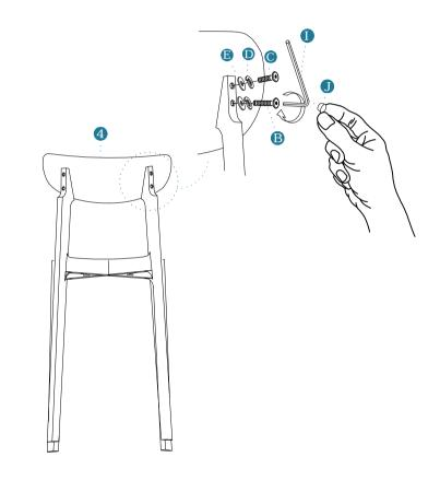
Attach 1 x backrest (4) to assembled frame and secure with 2 x screws (C) and 2 x screw (B), 4 x spring washers (D), 4 x washers (E). Please make sure you use screw (C) for the top hole and screw (B) for the bottom hole. Tighten with an Allen Key (I). Once tightened insert 4 x wood buttons (J) as shown
