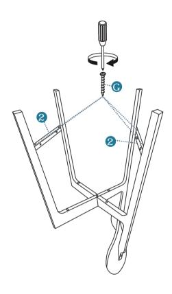
Attach 2 x rails (2) to assembled frame as shown and secure with 4 x screws (G). Tighten with a screwdriver.
