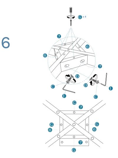
Each side has 2 x screws (C) and 2 x spring washer (D).
