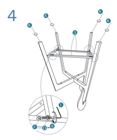
Attach 2 x support bars (3) to assembled frame, 4 x felt pads (K) as shown and secure with 4 x screw pins (F), 4 x spring washers (F) and 4 x screws (F). Tighten with an Allen Key (F).
