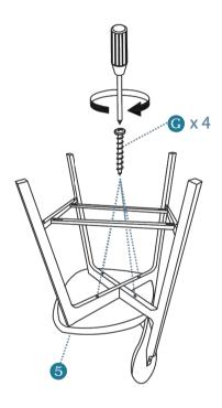
Attach the legs to the seat base with 4 x screws (G) as shown. Tighten with a screwdriver.
