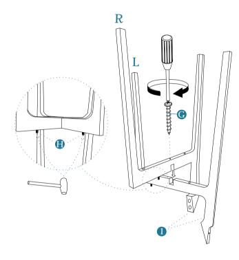
Attach 2 x legs (1) together as shown and secure with 1 x screw (G) and  $2 \times 1$  dowel (H). Tighten with a screwdriver.
